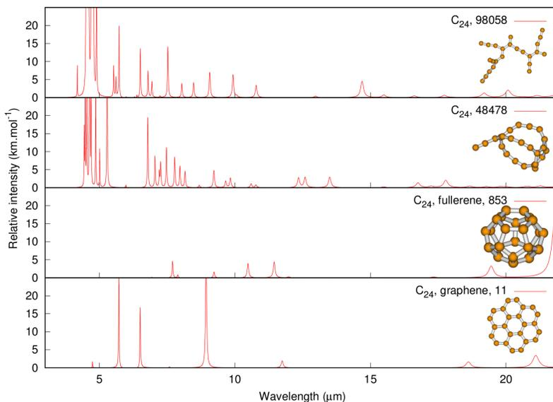
Figure 1: Examples of absorption IR spectra for optimized isomers of  $C_{24}$  at the SCC-DFTB level. A scaling of 0.84 on the vibrational energy is applied for wavelengths above  $6 \mu\text{m}$ .
