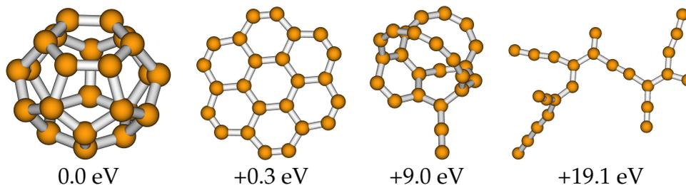
Figure 1: Examples of relaxed isomer of C<sub>24</sub> optimized at the SCC-DFTB level.
